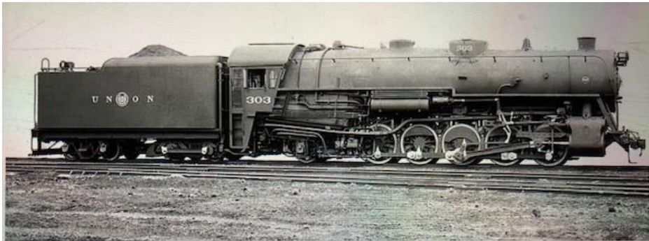
This profile view of Union 303 shows its immense size. It had 61-inch drivers and an 88-inch diameter boiler. Baldwin photo, Classic Trains collection
