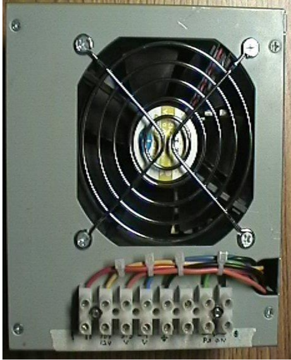
Figure 2. Fan and Terminal Strip.
