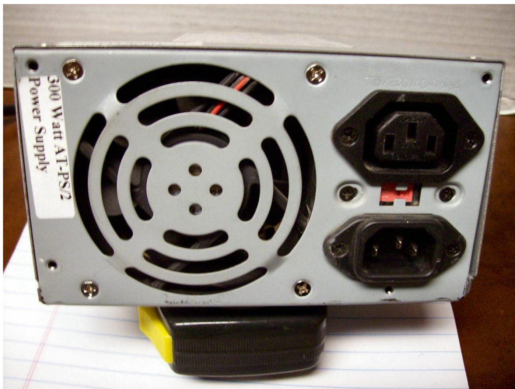
VIEW OF THE SPI-300 FRONT PANEL. The AC input connector is on the bottom right. The AC output connector is on the top right. The 12 volt cooling fan is on the left.
